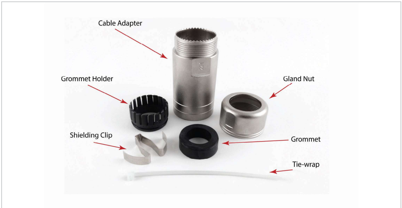
New Assembly Kit with Replacement EMI Shielding Clip
